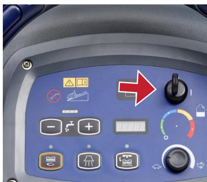
7. Turn on the key, then slightly press the handle switch to engage the brush.
