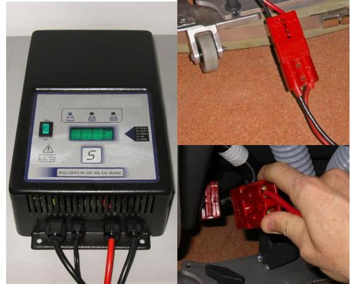
1a. Switch off charger by unplug charger cable from red battery plug. Reconnect the red battery plug to the machine.
