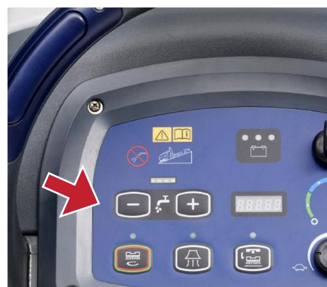
8. Adjust (if needed) the solution flow level according to the cleaning performance and application.
