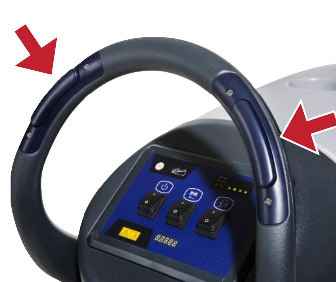
8. Press the handle switch to engage the brush and run the machine.
