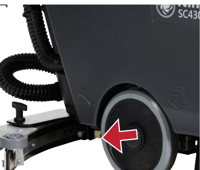
6. Adjust the eco solution flow control valve.
