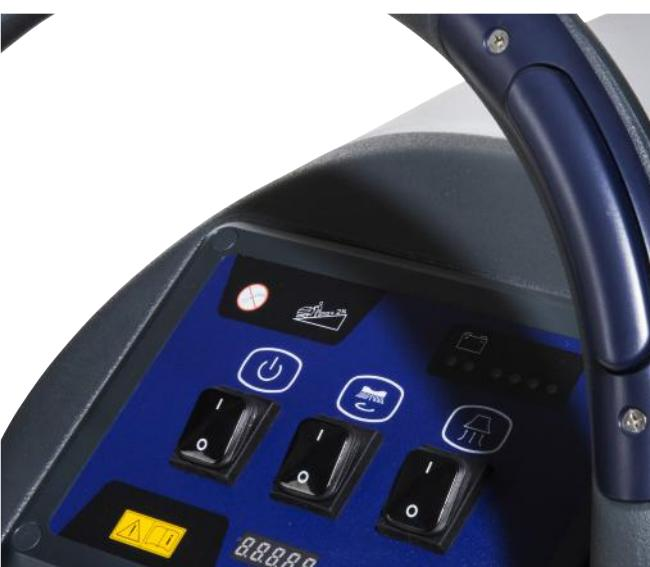
7. Switch on the brush and vac motors to activate the machine.
