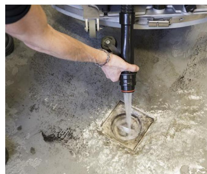
9. **At the end of the work.** Empty the recovery tank with the hose. Then empty the solution tank with the transparent hose.
