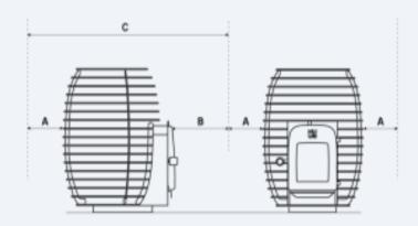
\* In case the HIVE Heat heater is installed near combustible material and necessary safety distance cannot be guaranteed, use a heat reflector to reduce the safety distance by half.
