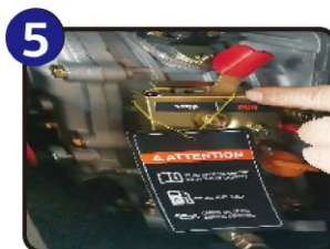
PULL THE SPEED CONTROL LEVER TO "RUN" POSITION.
